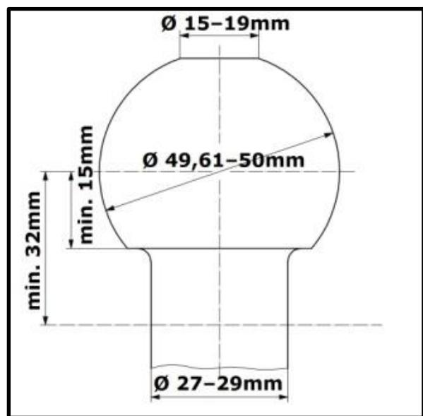
Fit the bike carrier only to trailer couplings with the following properties:
